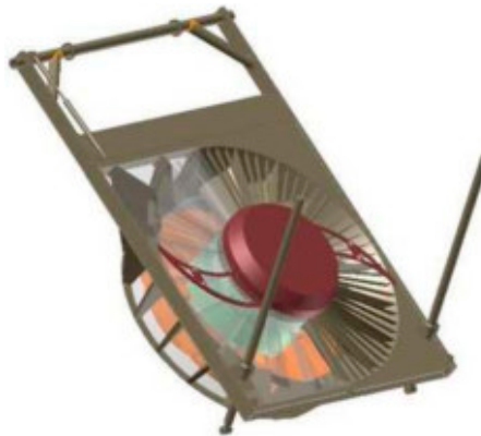
Figure 67. Front view of Very Low Head (VLH) turbine with its supporting structure.
