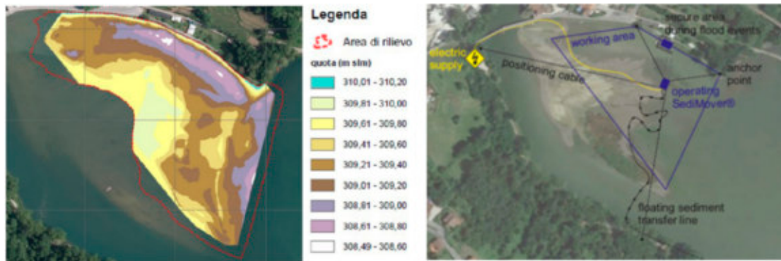
Figure 16. Results of the bathymetry to define the initial state of the sediment in Pontecosi and configuration of transfer line over the work area.
